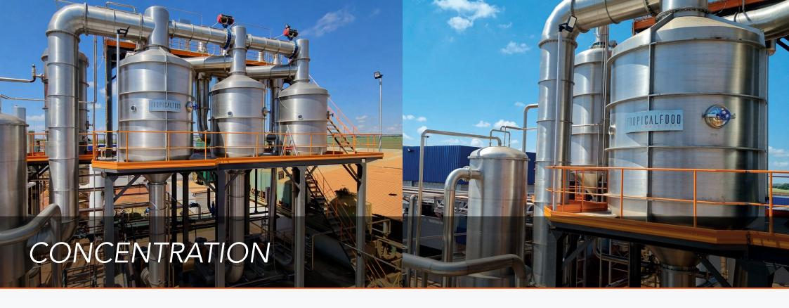
Our complete next-generation concentration lines meet the diverse demands of the market. All TropicalFood Machinery concentrators operate in triple concurrent thermal effect flow, with forced circulation through the ascending and descending tube bundle. With a capacity to process up to 1,500 tons/24h, our concentrators are ideal for producing high-density extracts, including crushed tomatoes.
