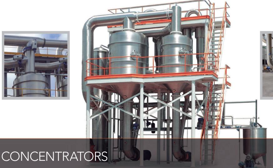
TFM manufactures processing lines for the concentration of fruit and tomato juices. These plants can handle capacities ranging from 500 up to 50,000 L/h of evaporated water, featuring multiple effects and different automation levels, from the simplest to the most advanced. Our concentrators are specially designed for high-consistency and high-viscosity products. Thanks to the short residence time, there is a significant improvement in the quality of the final product.
