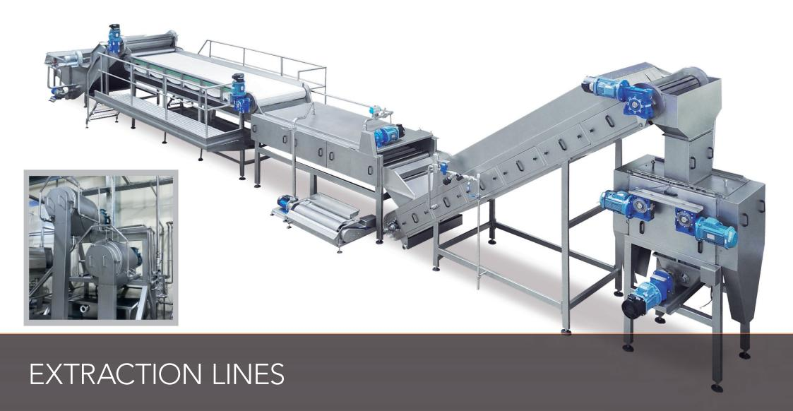
TFM designs and manufactures processing lines for the separation of the edible part of the fruit, both in manual and automatic modes, according to customer requirements and the type of fruit.
