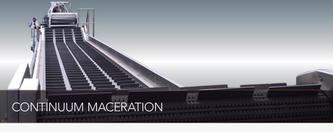
From the receipt, washing, and selection of the raw materials, the entire process is carried out continuously, including maceration and water dosage during the extraction phase. All equipment has speed control via frequency inverters to ensure there is no shortage or excess of product, maintaining a consistent process.
